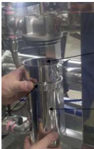
Figure 11: installing a pre-filter
