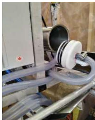
Figure 9.2: Membrane seal
