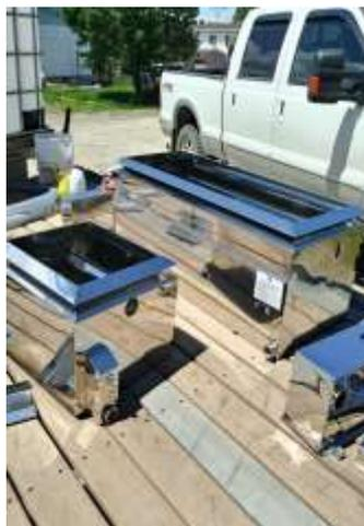
Figure 22.2: Evaporator parts being cleaned individually
