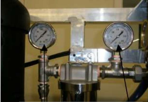
Figure 12: Sap pressure gauges
