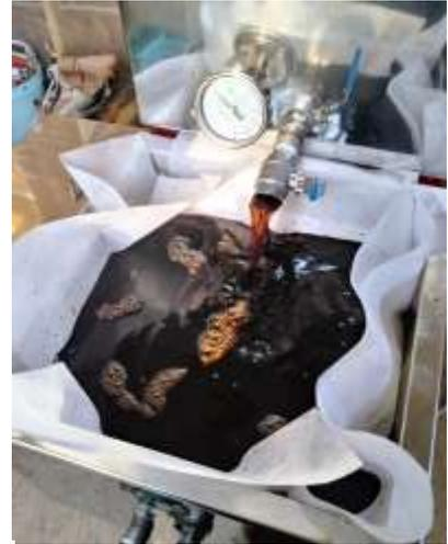
Figure 18.2: Syrup being filtered
