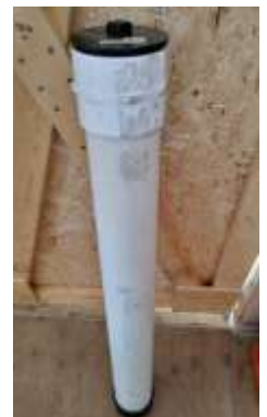
Figure 7: Membrane Storage Cylinder
