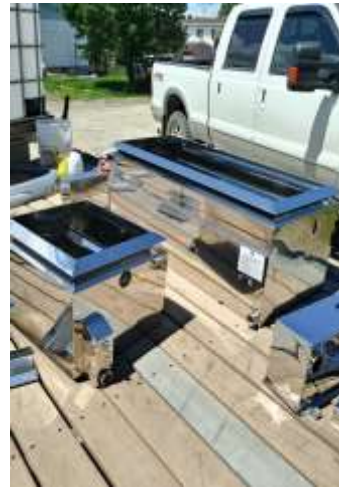
Figure 22.2: Evaporator parts being cleaned individually
