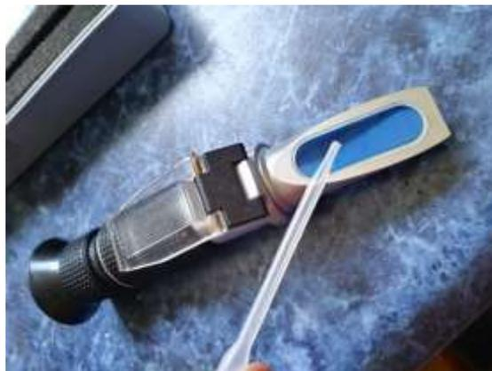
Figure 15.1: Refractometer
