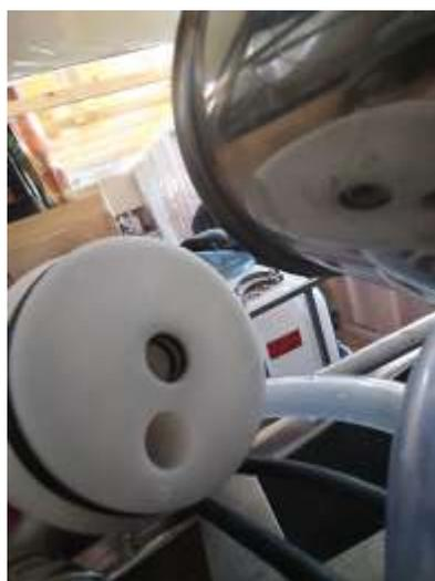
Figure 9.4: O'Rings inside membrane seal
